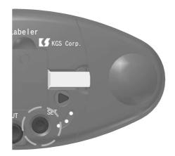
6. Push Cut Key and cut off printed tape.
