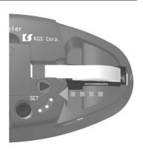
4. Push the Set key to arrange the position of an edge of a braille tape so as to be in right position before printing dots.
