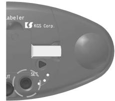
3. Push Cut Key and cut off printed tape.
